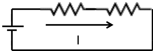
Resistors in Series Add Together
